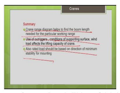
So, we saw the importance of crane range diagram. It will help you to find what is the boom length needed for a particular working range or what a working range boom length can offer. Either way, you can get the data from the crane range diagram. It helps to find the boom length needed for the particular working range. So, you should also always note that the crane rating given by the manufacturer is done.
