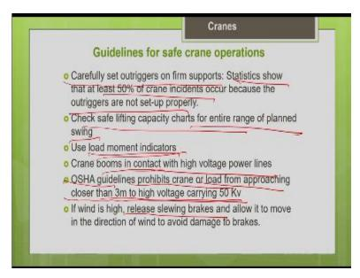
There are also some guidelines given for the safe crane operations because you know that there are so many accidents related to crane reported very commonly. So, that is why we should follow some safe guidelines when you operate the crane. So, carefully set the outriggers on firm supports because statistics shows that at least 50% of crane incidents occur because outriggers are not extended properly that is why we have to carefully set the outriggers and is also check for the soil condition.
