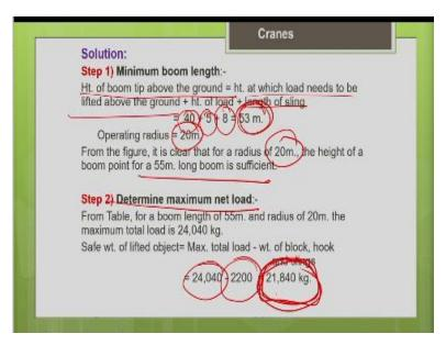
So, that is what is given here. The height of boom tip above the ground equal to height at which the load needs to be lifted above the ground, it is 40 meters. Height of the load is 5 meter plus the length of the sling is 8 meters. You add everything; you get 53 meter that should be the height of boom tip above the ground that is what you need for this particular project. And the operating radius, the horizontal radius is 20 meters.
