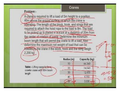
So, here, a crane is required to lift a load of 5-meter height. The height of the load is 5 meters to a position of 40 meters above the ground surface on which the crane is operating that means the lifting height needed is 40 meter above the ground. The lifting height needed is 40 meter above the ground and the length of the block hook and the slings that are required to attach the hoist rope to load is 8 meters. So, that is also provided to you what is the length of the block, hook, slings?
